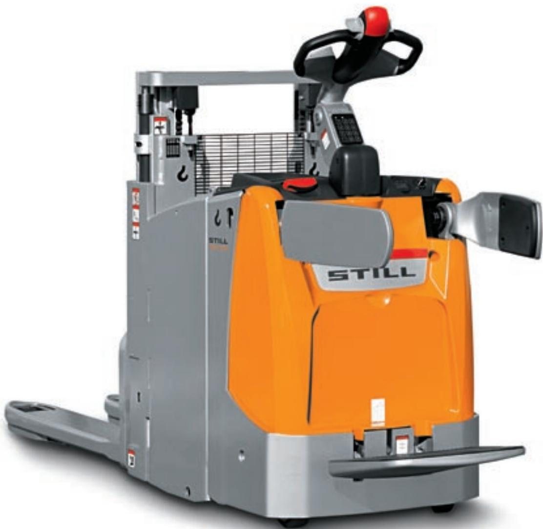
The EXD-S is a heavy-duty double decker high lift pallet truck that can lift a maximum of 2,000 kgs when using the initial lift or twice 1,000 kgs when utilising double decker loading and unloading. Two pallets can be transported simultaneously with the EXD-S - so time can be saved by the efficient loading and unloading of lorries.
