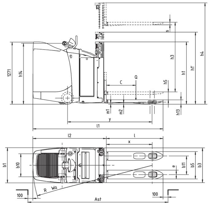
This specification sheet to VDI Guidelines 2198 or 3597 only gives the technical figures for the standard truck.
