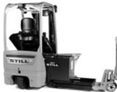
3) Battery change with a standard hand pallet truck, low lift truck or battery change frame
