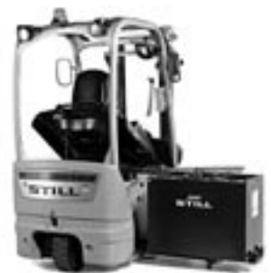
4) On-board roller platform for exchange by hoist
